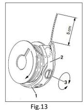
Insert the bobbin into the bobbin case 1 Pass the thread through the slot under spring 2. Pass the thread through the notch. Adjust the thread tension by turning screw 3.
