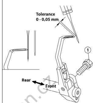
When tip of looper moves to the center of chain stitch needle, the tolerance between looper tip and needle grove should be 0-0.05 mm. Adjustment can be made by loosen screw (1).
