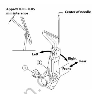
When lower Looper moves from right to left and the tip of looper moves to edging needle/right needle, there will have a interference approx 0.03 – 0.05 mm. Loosen screw (1) and adjustment can be made by moving looper arm (2) forward or backward.
