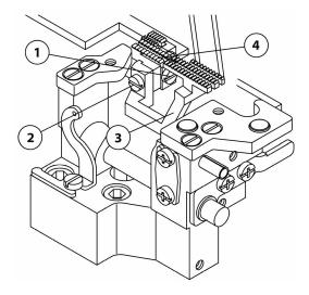
Loosen screw (1) can change main feed dog (4). Loosen screw (2) can change differential feed dog (3). After changed feed dogs, tighten screw lightly. Please refer to following items in order to set up correct position of feed dogs. Then, tighten set screw.
