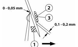
2. In the same time, adjusting rear needle guard (1) in order to push needle forward and create a tolerance of 0 - 0,05 mm between needle and the tip of lower looper.
