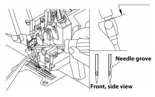
Make sure to insert needles all the way to the bottom of needles holes.
