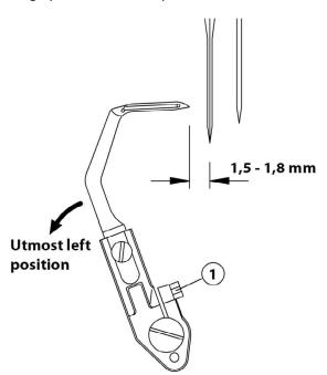
When chain stitch looper moves to its utmost left position, the distance between tip of chain stitch looper and the center of chain stitch needle should be 1,5 mm. Adjustment can be made by loosen screw (1).
