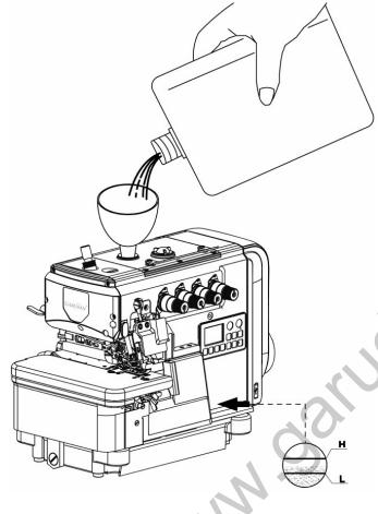
During adding process, please make sure the lubrication oil can't over the upper limit of oil gauge.
