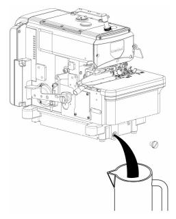
After operating sewing machine for 160-200 hours (approx one month) and please change lubrication oil and change lubrication oil every 6 months thereafter.
