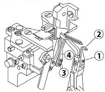
Please take off rear needle guard (2) by loosen set screw (1). Loosen set screw (3) can take off front needle guard (4).
