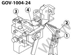
Can take off rear needle guard (2) by loosen screw (1). Loosen screw (3) can take off front needle guard (4).
