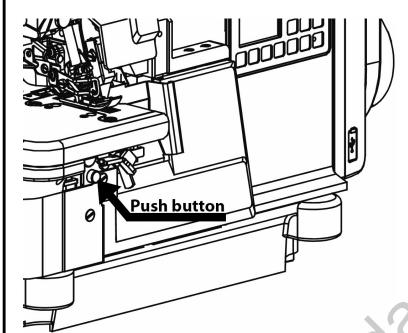
Pushing the push button lightly first and turning pulley to set position then pushing down the push button into its set position and adjust the length of stitch.
