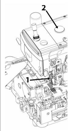
The distance between needle tip to top of needle plate should be 10 mm (standard setting).
