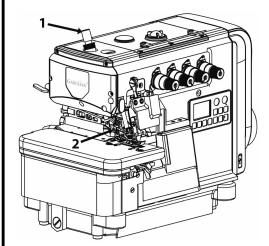
Turning adjusting screw (1) counterclockwise in order to loose pressure spring. Loosen screw (2) can take-off presser foot set.
