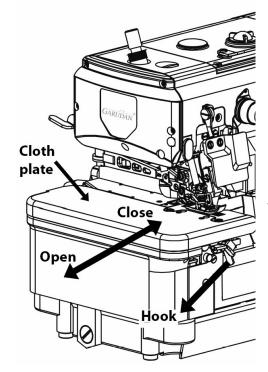
Press down hook and push to left in order to open cloth plate, pushing right to its hook set position, the cloth plate will be close.
