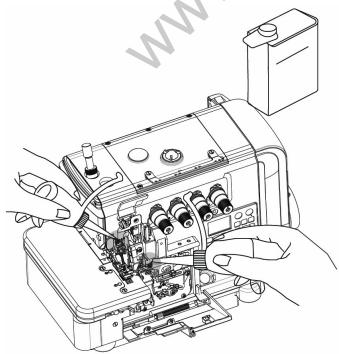
Please add proper silicon oil into silicon oil reservoirs in order to prevent thread breakage.
