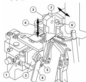
Loosen screw (1), push lower knife holder (2) to left and then tighten screw (1) lightly.
