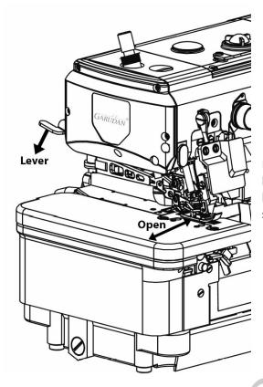
Push the lever down and then pull out the foot of the hanger. To return to its original position, push the lever downwards and retract the shoulder arm. Make sure the foot is in the correct position.
