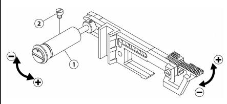
During feed dogs movement, the teeth of feed dogs must be level off always. Adjusting its level or during some special requirements, feed dog teeth must tilt to front or rear.
