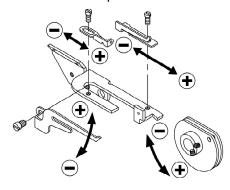
When adjusting chain stitch looper thread, if thread loop collapse, unstable or can't form thread loop, please adjust thread tension amount.
