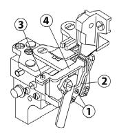
Loosen set screw (1) can take off rear chain stitch needle guard (2). Loosen set screw (3) can take off front chain stitch needle guard (4).
