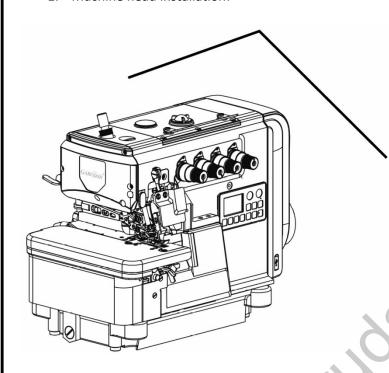
Please make sure there have enough room between sewing machine and the table around it after installation. Table can't interference with the sewing machine.
