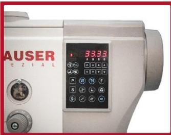
Integrated 750W sewing drive with on-board control panel. Power consumption 0,7kVA
