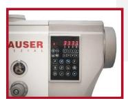
750W Integrated sewing drive with on-board control Power panel. consumption 0,7kVA
